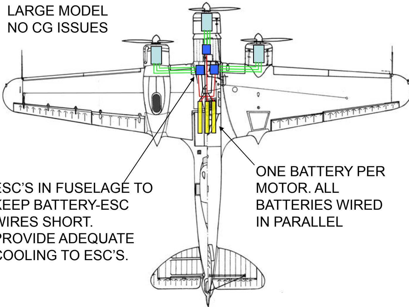
ESC'S IN FUSELAGE TO
